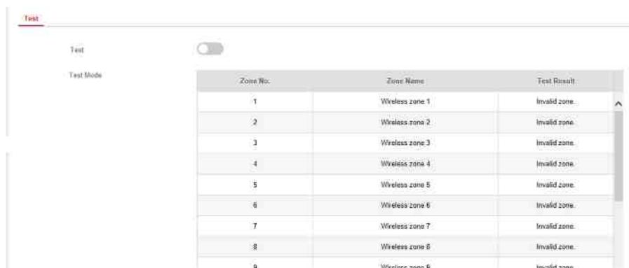
2. Check the **Test** check box to start walk test.
